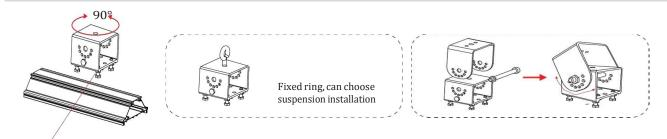
Square symmetrical design with four corners, can be rotated 90°horizontally or vertically
